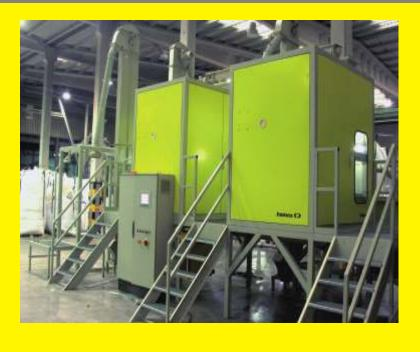
hamos EKS Electrostatic Separators separate mixed plastics in a dry process achieving very clean plastic fractions with a low running cost. Mixtures of PS/ABS, PVC/rubber, HDPE/PP, PET/PVC, PP/PS, ABS/PMMA, PVC/PE and many more can be successfully separated. The EKS works independent from colour and separates mixtures of black plastics as well. For the separation to be successful, the material must be dry, dust-free and < 10 - 12 mm.
