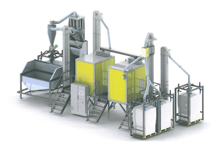
The illustration shows an example of a **hamos EKS-PET** turnkey system for high throughput rates with fully automatic material handling. The line is designed for 24/7 operation.
