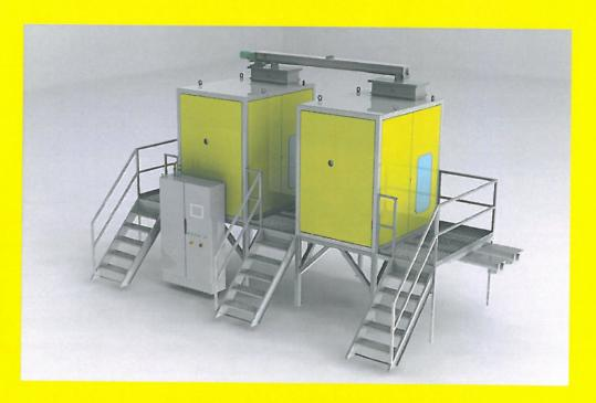
The **hamos EKS-PET** electrostatic plastics separators separate undesired PVC and other contamination like shrink sleeve labels made of PETG or other thermoforms from PET flakes, to produce a clean PET fraction. Due to its working principle the **hamos EKS-PET** separates other materials as well. The separation process works in a dry manner with low running cost.
