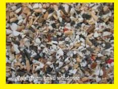
The **hamos WRS** recycling line has been conceived specially for processing of PVC window profiles. Regrind material from both production waste as well as used windows can be recycled. The PVC has such high purity after separation that it can be directly processed again by coextrusion into new profiles.
